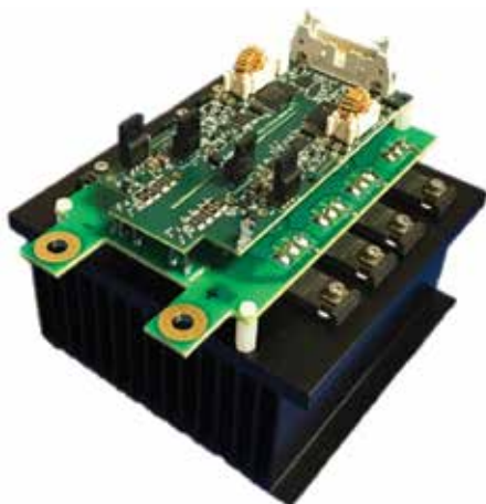
The Gate Driver is mounted to a daughtercard which in-turn connects to the Power Devices.
