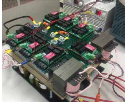
Three-phase three-level AC-DC-AC 20 kW, 480 V, 800 V DC, SiC-based UPS module with integrated three-level DC-DC battery charger under test.
