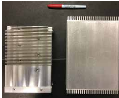
GaN charger (left), 4 kW/L vs. SiC charger (right), 3.3 kW/L.
