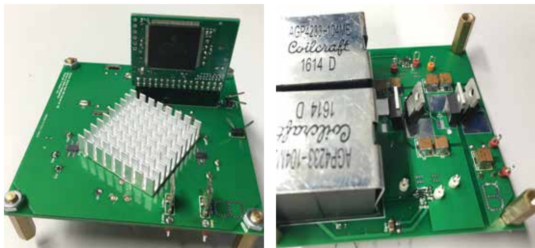
DCP HVG Converter (Left: Top; Right: Bottom)
