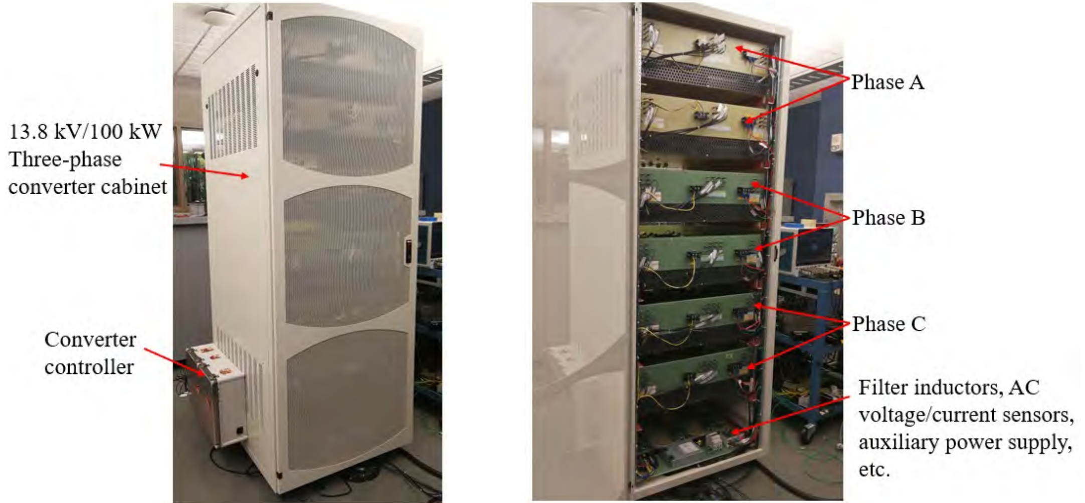
Three-phase PCS converter hardware pictures
