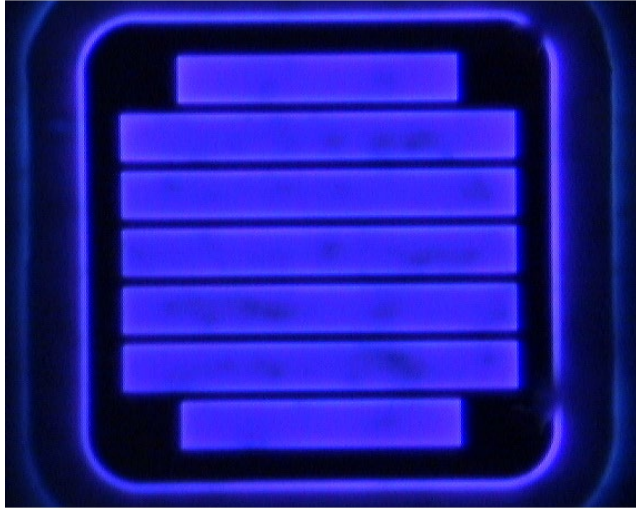
Gridded PiN Diode (ca 2006) EL image
