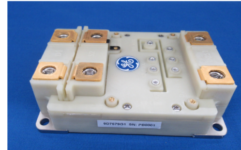
Baseline structure from GE's 3.3kV 1/2 Bridge Module
