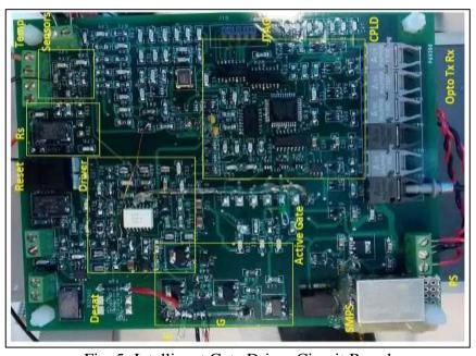
Fig. 5: Intelligent Gate Driver Circuit Board
