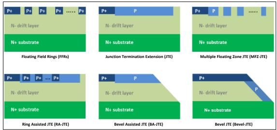
Fig. 1. Edge termination structures for high voltage SiC devices.
