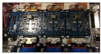
Figure 6: SiC dual inverter manufactured using PowerEx module, JDES Sic gate driver and film capacitor module
