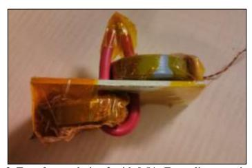
Fig.3. Transformer design 2 with 0.54 pF coupling capacitance
