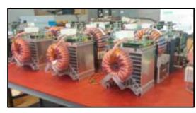
Fig. 7. EV fast charger prototype in develpment.
