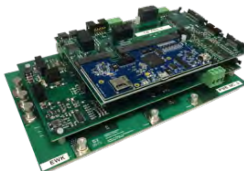
Basic building block (BBB) of the multiport power converter (MPC). From top: Control board, Gate driver board, Power board.
