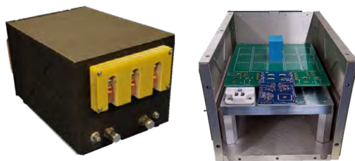
View of the 100kW 600 V GRU: (left) GRU enclosure; (right) internal view depicting cold-plate, SiC modules, gate-drive, PCB-based DC-bus.
