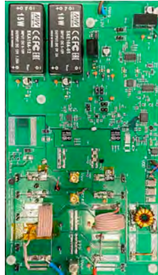
Left: Prototype Board with GS66508B GaN switch and variable capacitive network. Right: Class E/EF 2 -inverters applied in a wireless charging system.
